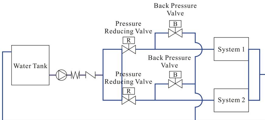
© In different pressure systems of processing pipelines, installing back pressure valve can maintain required pressure of the systems and ensure safe uses of equipments after pressure reducing valve reduces pressure.
