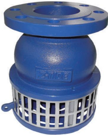
Foot valve is for use as inlet of suction pipe. A modified check valve that has a screen on the suction end to prevent debris from entering the pump or pipe. It protects against loss of prime, aids in priming the pump and protects the pump from large debris. (Only Vertical installation)
