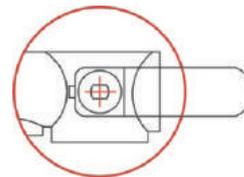
When the handle is rotated to horizontal position, pressure reducing valve set becomes bypass open state.
