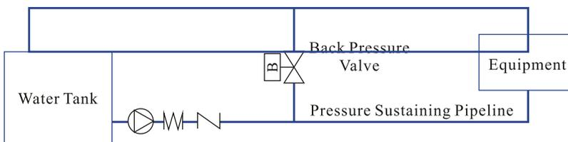
© Installing back pressure valve enables largest flow application and also stabilize pipeline pressure.
