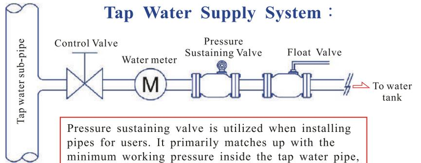
Pressure sustaining valve is utilized when installing pipes for users. It primarily matches up with the minimum working pressure inside the tap water pipe, balancing up-stream and down-stream pressure during normalcy and emergency, and maintains constant pressure inside the pipe.
