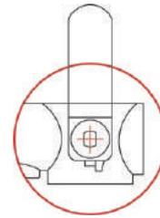
When the handle is rotated upward, pressure reducing valve set becomes pressure reducing open state.
