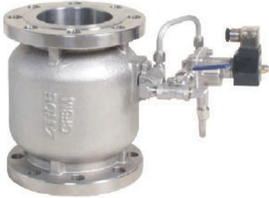
▶ Solenoid control valve is a kind of isolation valve, which can substitute traditional gate valves, ball valves and butterfly valves. The gate functioning is easily controlled by electrical power. The valve can be installed in fire control facility, water supply, or distant location where it's difficult to control the gate opening. The controller is directly fixed and can be easily installed on piping site. Interchangeable between manual and solenoid control.
