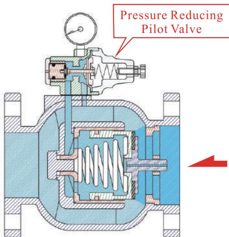
The pressure reducing valve uses a sub-valve (pressure reducing pilot valve) to control the main valve. When the outlet pressure reaches the setting range of pressure reducing pilot valve, the pilot valve will automatically sense the outlet pressure and adjust the pressure of the back pressure chamber in the main valve, so the valve gate can be opened and consequently maintains the outlet pressure.
