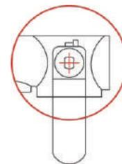
When the handle is rotated downward, pressure reducing valve set becomes pressure reducing closed state.
